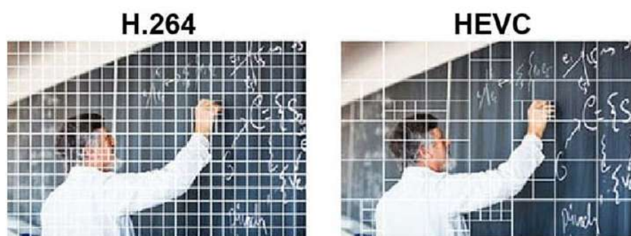
Figure 5.8 – H.265 (HEVC) and H.264 algorithm comparison
